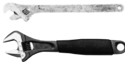
Johan Petter Johansson's adjustable wrench in its original 1892 design and in 1992, after a century of refinements.
